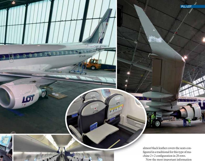
of almost 29 metres, it occupied almost the whole width of the hangar. It was also much longer than B 737 standing nearby. The total height of the aircraft is impressive 10.55 m. The new Embraer is powered by two CF34-10E engines manufactured by General Electric. Each of them measures 1450 mm in diameter and weighs 1678 kilograms.
