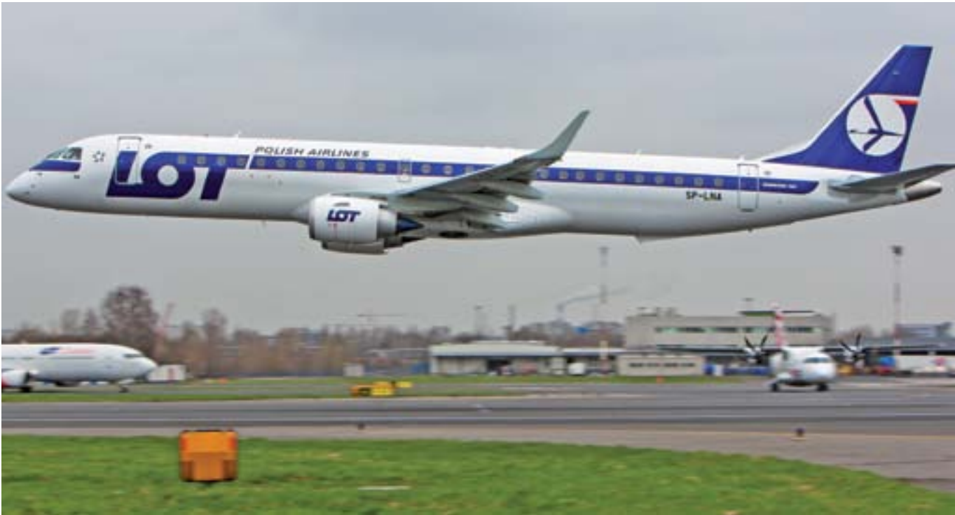
Embraer 195 is a medium-range aircraft (2,600 km) with a maximum cruising speed of 890 km/h. It's 38.65 m long and has a wingspan of 28.72 m. It can seat up to 112 passengers.
